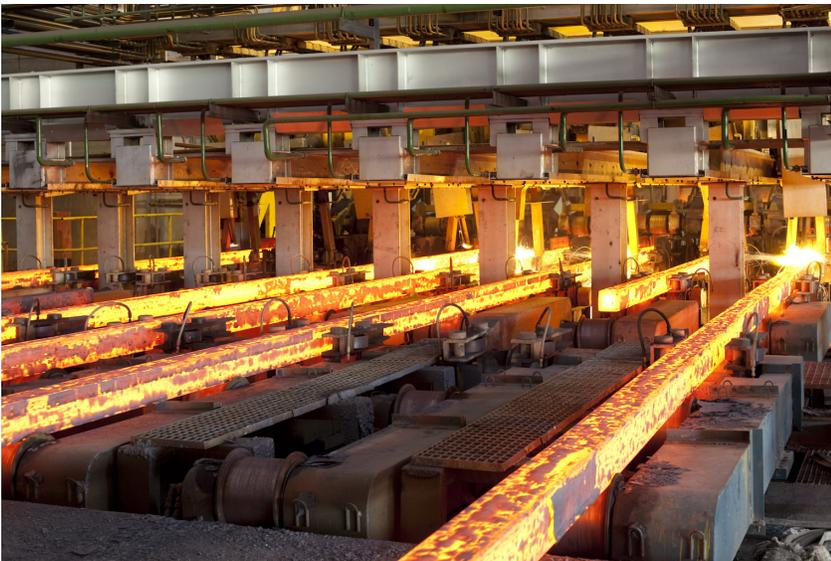
High-speed casting in eight strands on an SMS Concast casting machine.
