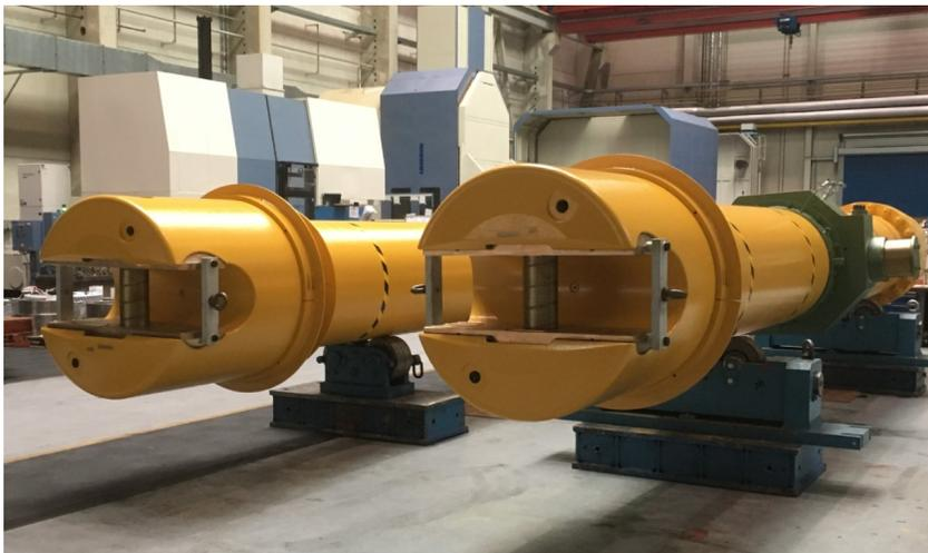
The SMS flat-neck spindles guarantee the safe and efficient transmission even of extremely high torques. (Photo taken during the workshop assembly).
