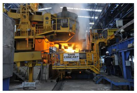
Casting of steel on the new continuous billet caster of SMS Concast assures BISW in Bangkok a high production output.
