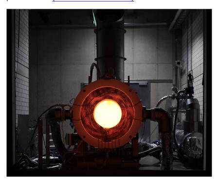
Solar receiver by SMS group's new partner Synhelion: delivery of clean solar process heat beyond 1,500 degree Celsius applicable to various industries using high-temperature process heat.
