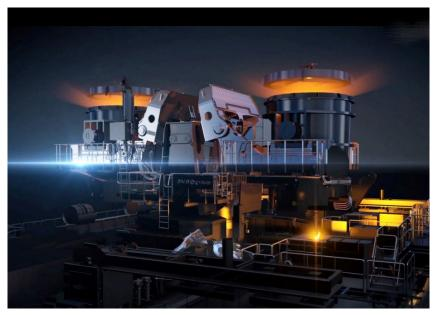
Casting platform of the new continuous slab caster at Nucor in Brandenburg, Kentucky, USA.
