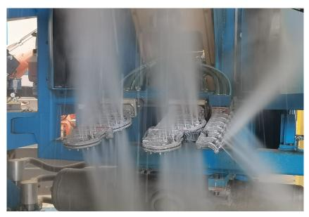
In action: the die lubrication system with additively manufactured spray heads.
