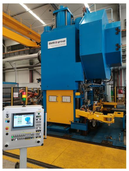
The new, fully automatic 2,500-ton closed-die forging line from SMS group at Ningbo Xusheng Auto Technology. The die lubrication system features innovative, 3D-printed spray heads.
