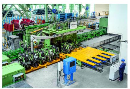
Reference picture of an SMS group  $\mathsf{PSM}^{\circledR}$  (Precision Sizing Mill).
