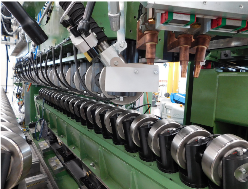
Detail view of the three-roller bending unit of the pipe forming station supplied by SMS.
