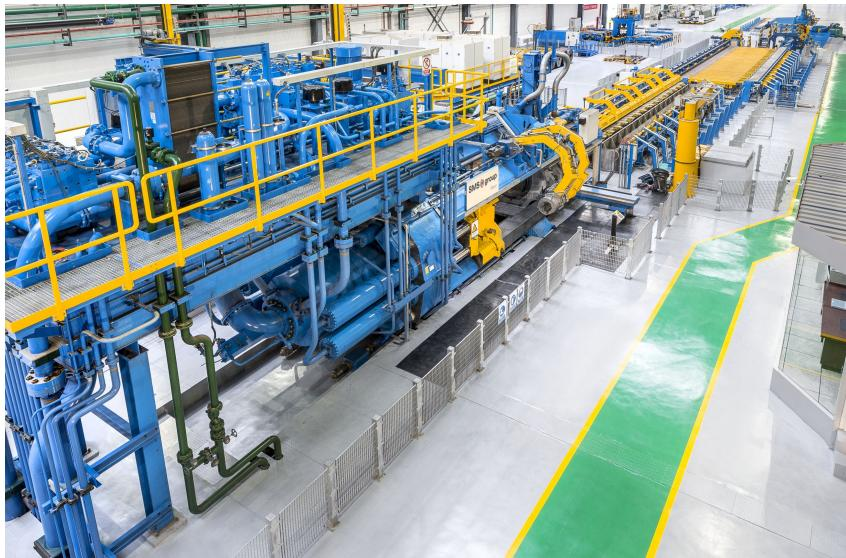
WEM uses the 45-MN heavy-metal extrusion press from SMS to produce zirconium mother tubes.
