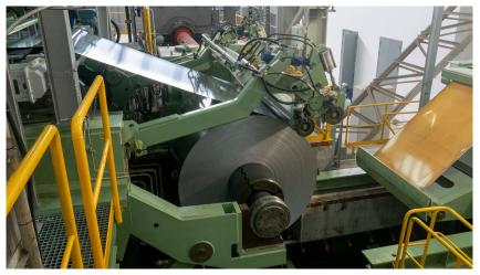
The first strip had a width of 1,780 millimeters and was rolled to a final gauge of 2.8 millimeters.
