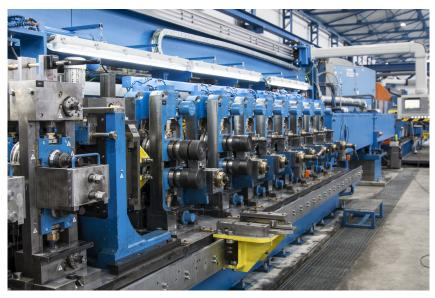
The 8-stand sizing section of Bornay's tube welding line from SMS group.
