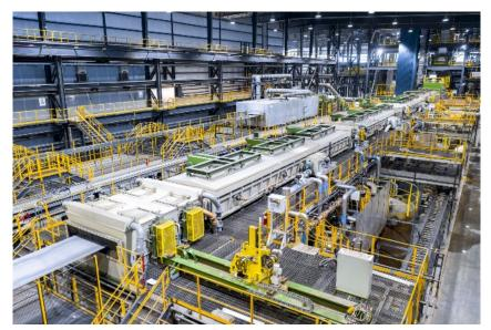
The U-shaped line combines turbulence pickling technology, high-power inductors, FOEN® galvanizing equipment and a Drever after-pot cooling system.
