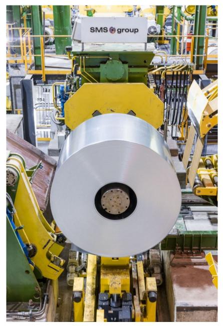
The "heat-to-coat" process permits the production of galvanized steel strip with durable corrosion protection, an appealing visual appearance, as well as an increased mechanical load-capacity while still maintaining low production and investment costs.
