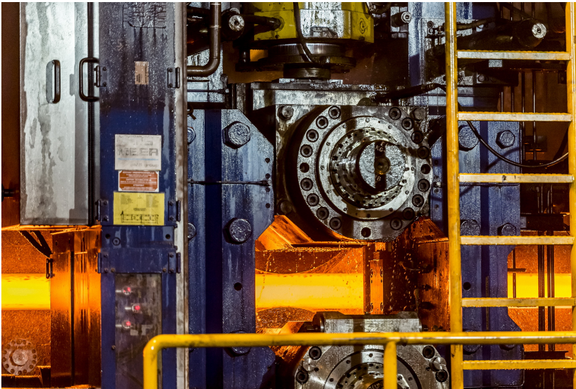
Close-up view of a break down mill stand built by SMS group.
