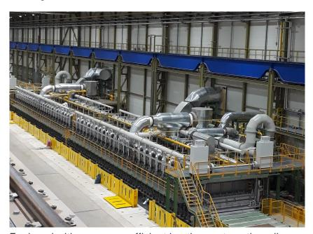
Equipped with an energy-efficient heating system, the roller hearth furnace supplied by SMS group is characterized by low emissions.
