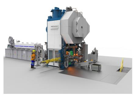
Fully automatic 25-MN forging line with automatic walking beam system, die spraying unit and die holder, and ELO-FORGE L induction heating system.
