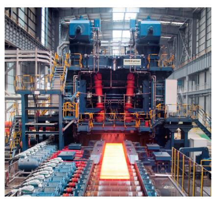
The second roughing mill rolls the slab in reversing mode down to transfer bar thickness. The attached edger ensures tight width tolerances and, as a result, high yield. The new high-performance hot strip mill supplied by SMS group has successfully started production at HBIS Laoting Iron & Steel Co. Ltd. in China. With this facility, HBIS Group, a leading steel producer in China, has set up a new, ultra-modern production facility for flat products at the Laoting location.
