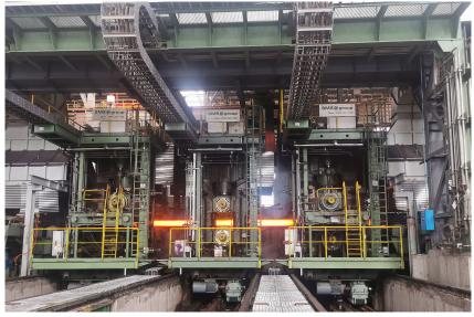
The centerpiece of the plant: the CCS<sup>®</sup> (Compact Cartridge Stand) tandem rolling mill unit with hydraulic adjustment system and fully automatic quick program change function.
