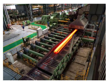
On the new heavy-beam mill, Masteel can produce beams with a maximum root face thickness of 1,100 millimeters and a flange width of 500 millimeters.
