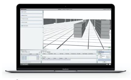
X-Pact<sup>®</sup> MES 4.0 Warehouse Management System for slab yard management allows to display the stored slabs in 3D.
