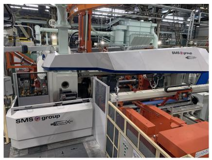
The new extrusion line supplied by SMS group to UACJ Extrusion Nagoya Corporation's for the facility in Nagoya, Japan: the HybrEx<sup>®</sup>40 press is the central unit of the line.
