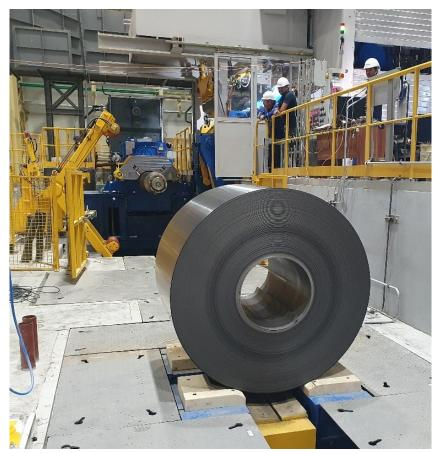
On August 6, 2020, the new RCM rolled the first cold strip to a final thickness of 0.45 millimeters in seven passes.
