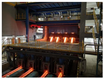
First cast of 255 x 300 millimeter blooms at Nanjing Iron & Steel Group Ltd. on the caster modernized by SMS Concast.
