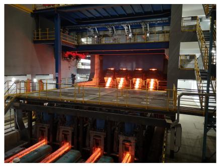
First cast of 255 x 300 millimeter blooms at Nanjing Iron & Steel Group Ltd. on the caster modernized by SMS Concast.
