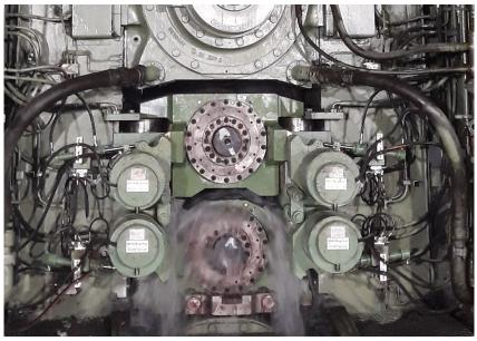
Finishing stand F4 of Wuhan Iron & Steel's hot strip mill after the installation of the  ${\rm CVC}^{\rm @}{\rm plus}$  system.
