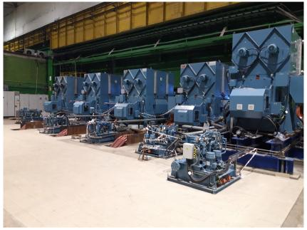
The new main drives for the mill stands: The main drive for the first stand had already been replaced in phase 1. In phase 2, the new drive for the tension reel was installed. The mill stands two, three and four received new main drives in phase 3.
