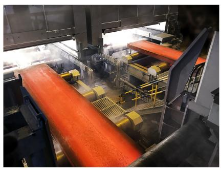
Casting of the first slabs following the successful revamp of the casting machine by SMS group.
