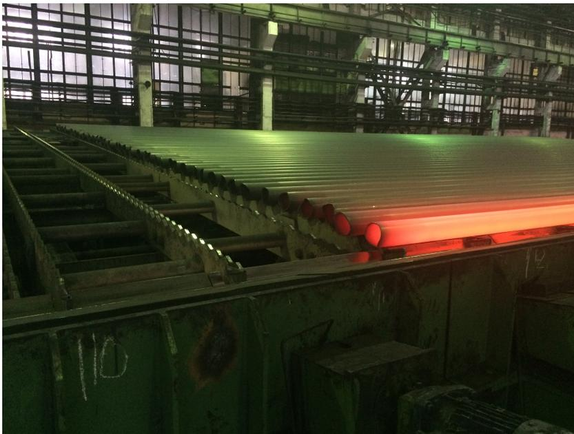
Seamless steel pipes on the cooling bed in the Tagmet PQF<sup>®</sup> mill.
