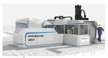
New Hybr $\text{Ex}^{\text{\tiny{B}}}$ 35 extrusion press with soundproof enclosure from SMS group.
