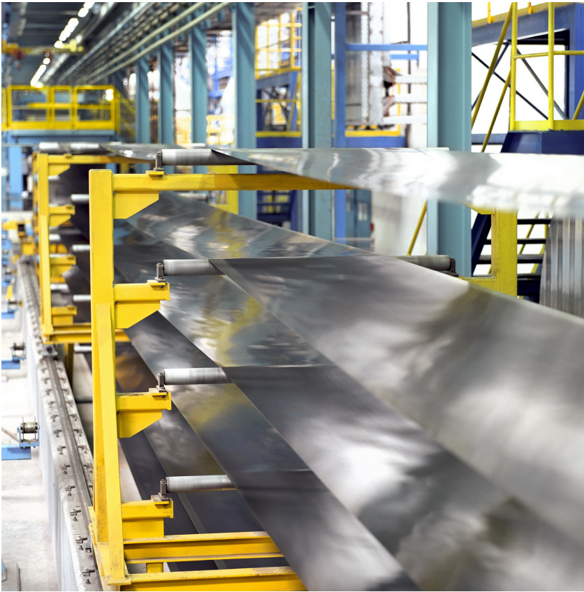
Horizontal strip looper in an annealing and coating line for non-grain-oriented electric steel strip.
