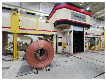
Specialized in rolling copper and copper-alloy strips of thick gauges: The new 4-high cold rolling mill of Jintian Ningbo Copper Co., Ltd.
