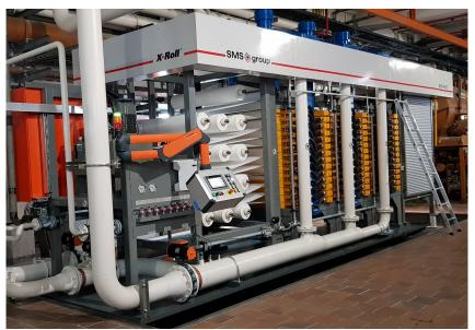
Final assembly of the Multi-Plate<sup>®</sup> filters at Hydro.
