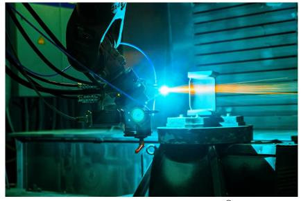
The thermal spraying system -  $\mathsf{PERFECT}$   $\mathsf{spray}^{\text{\'e}}$  -  $\mathsf{enhances}$  corrosion protection, not only of tubes.
