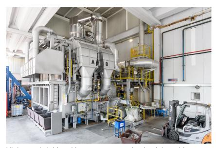
High metal yield and low energy costs in aluminium chip recycling at Cromodora Wheels thanks to the new chip melting furnace supplied by Hertwich Engineering.
