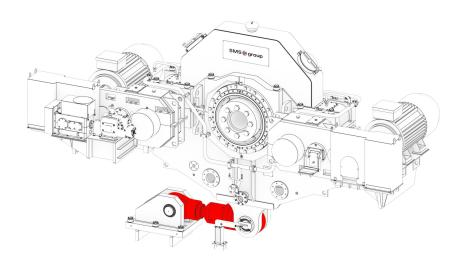
Gear unit of an AOD converter with vertical torque retainer from SMS group.
