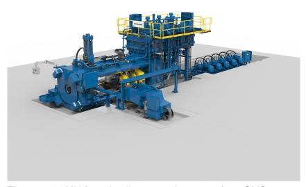
The new 45-MN front-loading extrusion press from SMS group.
