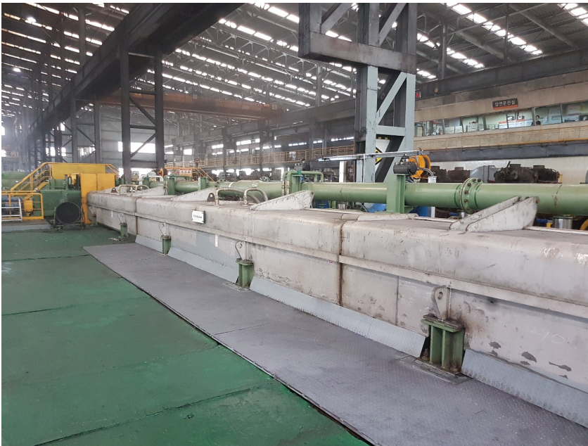
Rebar quenching system - water cooling boxes.
