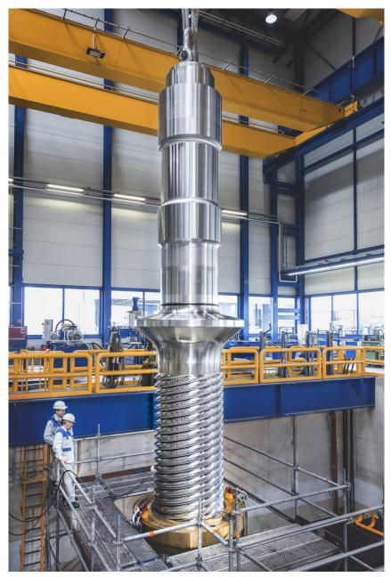
Perfect teamwork: the joining of screw and nut for the SPKA manufactured by SMS group in Mönchengladbach for AVIC Shaanxi Hongyuan Aviation Forging.
