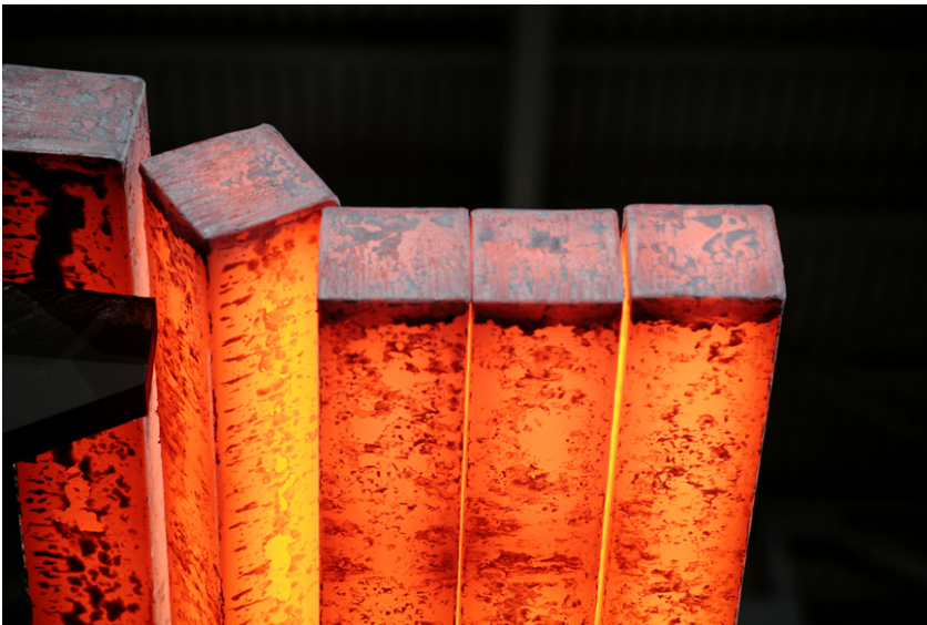
Billets produced on an SMS Concast caster.
