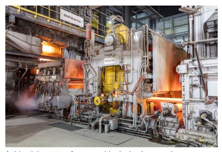
A thin-slab caster of comparable design in operation.
