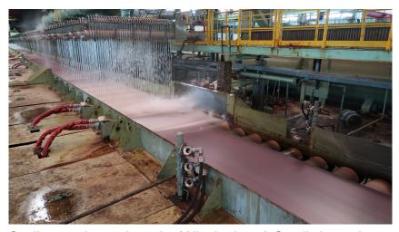
Cooling section at the exit of Ningbo Iron & Steel's hot strip mill modernized by SMS group. View of the reinforced laminar cooling and cross spray systems.
