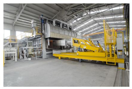
Multi-chamber melting furnace with preheat ramp (Ecomelt PR) from Hertwich (similar plant).
