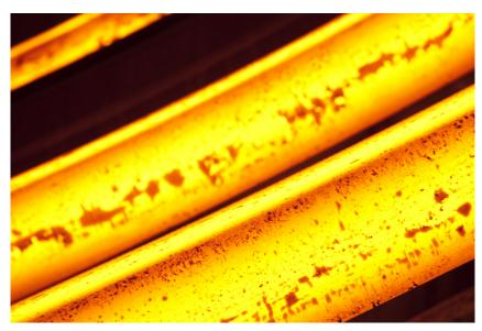
Rectangular blooms cast on a continuous caster made by SMS Concast.
