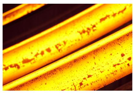
Rectangular blooms cast on a continuous caster made by SMS Concast.
