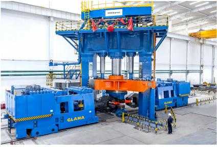
The new 63/80-MN high-speed open-die forging press in operation at WST.
