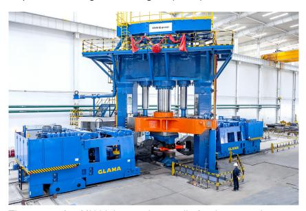
The new 63/80-MN high-speed open-die forging press in operation at WST.
