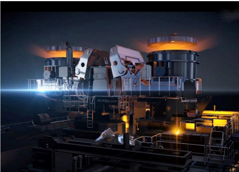
Casting platform of the new continuous slab caster at Nucor in Brandenburg, Kentucky, USA.
