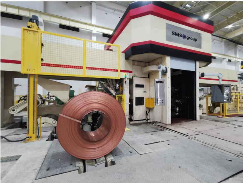
Specialized in rolling copper and copper-alloy strips of thick gauges: The new 4-high cold rolling mill of Jintian Ningbo Copper Co., Ltd.
