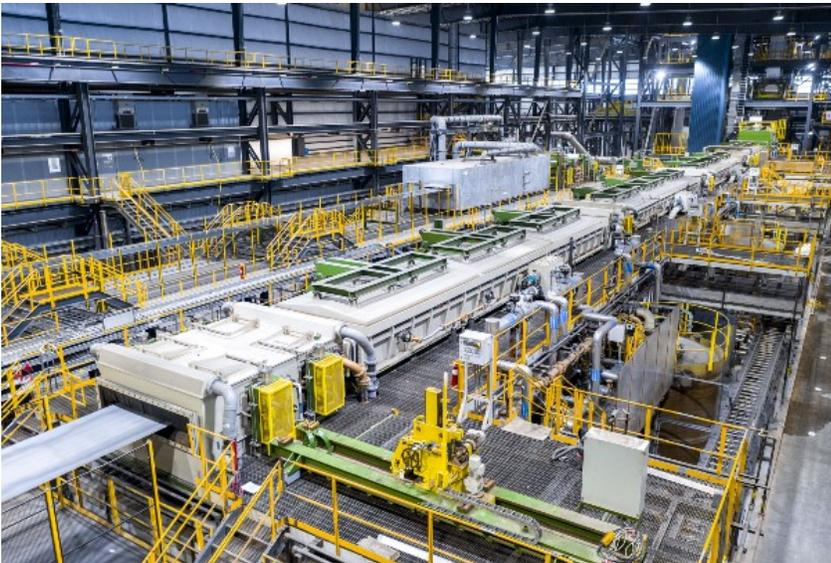
The U-shaped line combines turbulence pickling technology, high-power inductors, FOEN<sup>®</sup> galvanizing equipment and a Drever after-pot cooling system.
