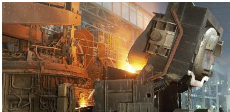
Hot metal charging
