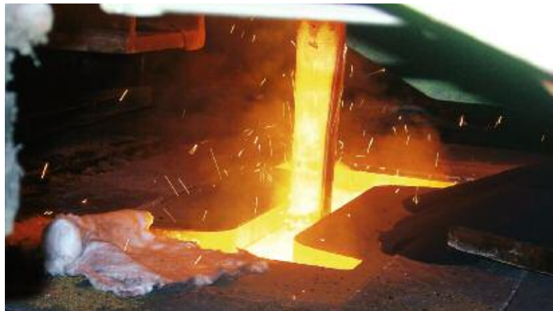
Casting of the widest beam blank
